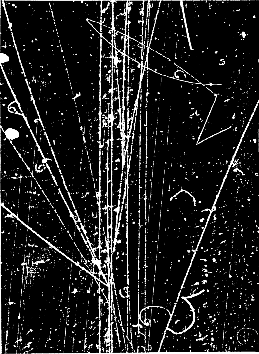
Fig.1. A four-prong Q = +4 star with associated fast and slow V^0 -particles and a low energy \gamma -quantum, produced in p^{12}\text{C} collision at 10 GeV/c
